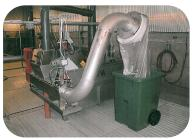
Solid Waste separator container is used for mechanical removal of sludge. SWSC consists of a screen and a Screw Wash Press, which is mounted on the outside of the tank. A sand conveyor is installed in the system. Further, the equipment has a built-in sedimentation tank that separates gravel and stones from the sludge, before it reaches the fine screen.
