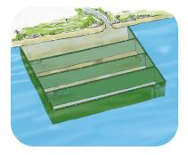
Floating log diameter 20 cm deep maximum 1,5 meter. Wall length and depth are different for each project, the walls are mounted with a chain at the bottom (chain weight 5,6 Kg/meter. Concrete weights 52 Pc a 40 Kg for side positioning of the floating walls to be placed on the liner. The weights have cushions not to damage the liner. Järven Floating wall will increase the detention time an give the pond a optimised hydraulic condition.
